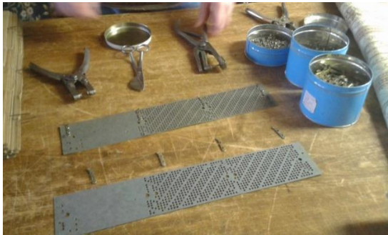
Figure 16: Single punch cards /one punch card =one weft
