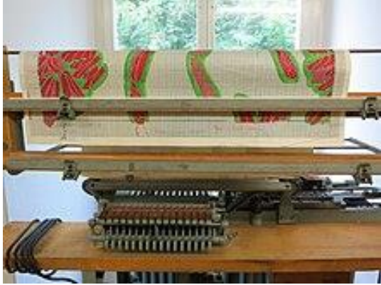
Figure 15: Cartridge mounted on card punching machine
