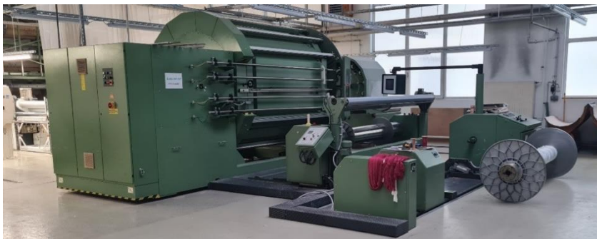
Figure 25: Modern warping machine
