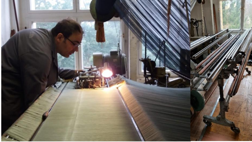
Figure 28: A warp-tying machine
