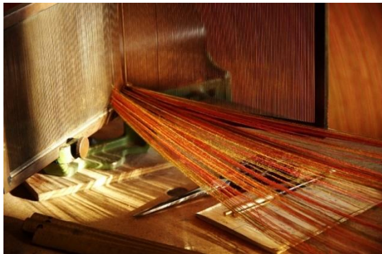
Figure 15: Reed examples. The photo is owned by the company Texulting GmbH .
