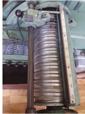
Figure 15: Reed examples. The photo is owned by the company Texulting GmbH .
