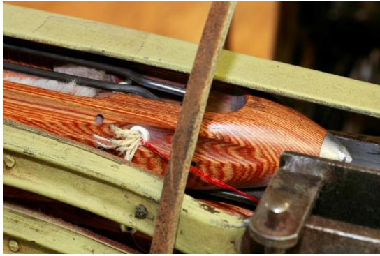
Figure 20: Shuttle with weft thread. The photo is owned by the company Texulting GmbH.
