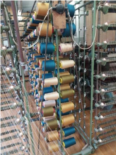
Figure 13: Historical warping gate. The photo is owned by the company Texulting GmbH .
