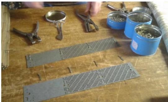
Figure 6: Single punch cards /one punch card =one weft. The photo is owned by the company Textulting GmbH.
