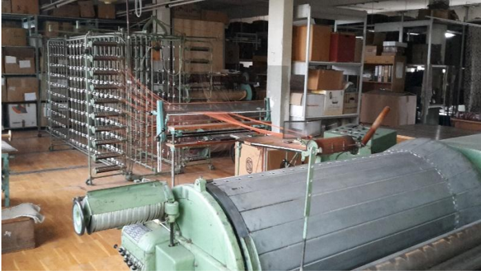
Figure 12: Warping machine. The photo is owned by the company Texulting GmbH .
