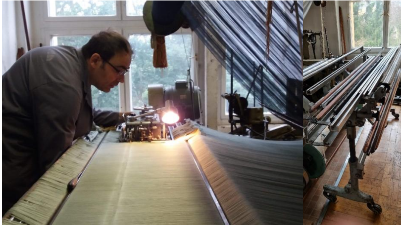
Figure 19: A warp-tying machine. The photo is owned by the company Texulting GmbH.
