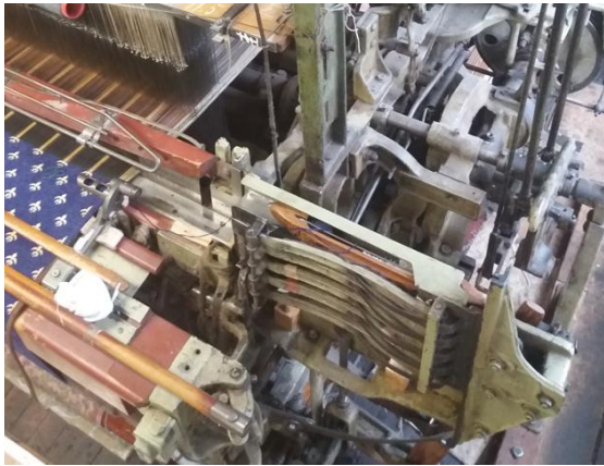
Figure 21: Manual Shuttle box. The photo is owned by the company Texulting GmbH.
