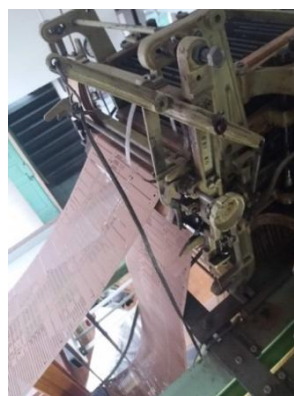
Figure 9: Jacquard attachment. The photo is owned by the company Textulting GmbH.
