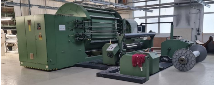
Figure 16: Modern warping machine. The photo is owned by the company Texulting GmbH.
