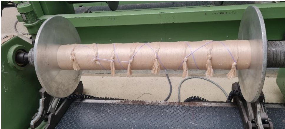
Figure 17: Warp beam. The photo is owned by the company Texulting GmbH.
