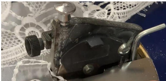
Figure 8: Knife to cut embroidery borders. Image is owned by the company Textulting GmbH.
